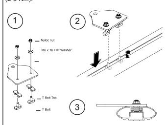
Assemble hardware and light bracket as detailed below. Locate the channel nuts into the crossbar recess, turn the bolt so that the channel nut rotates and locates as shown. Adjust to desired position and tighten bolt securely (2-3 Nm).
