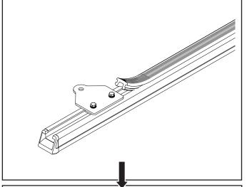
Mount work light onto the bracket.
